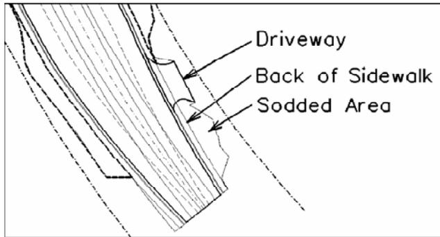
3. Create a closed feature for the area shown as Sod in the sketch above. Select **Quantities > Shapes Tool**, toggle Shape mode to **Fill**. Verify that the Surface is "Proposed with Drive". For Feature Name, key-in "Sodding". Set the Feature style to "Grassed Areas". Turn on the Dynamics toggle and Apply.
