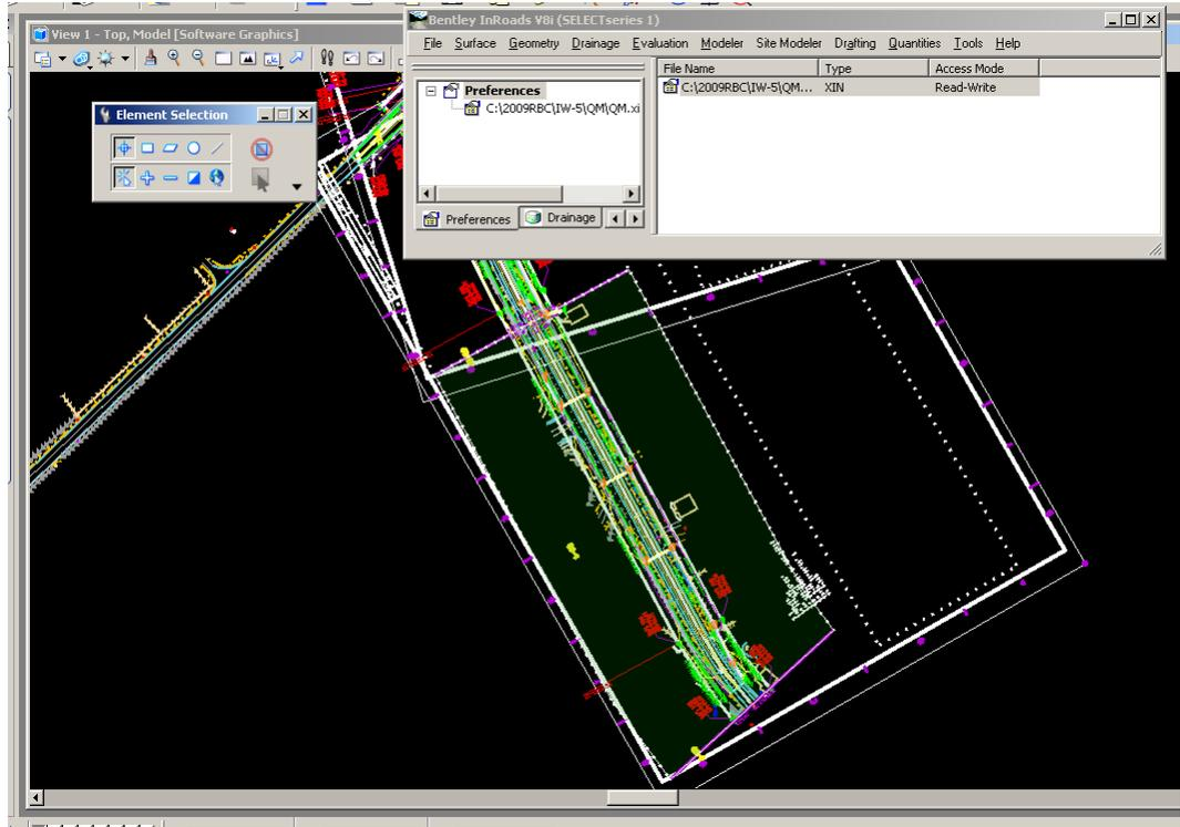
3. Place a Fence using the by Element method for the first (southernmost) sheet in the plan assembly. Set the Fence Mode to Clip.
