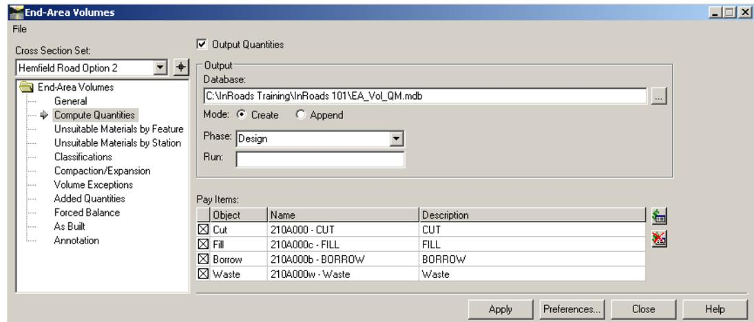
Select “Output Quantities” and specify the Output database (use the working directory – NOT the sample indicated above). Note – for this portion, we are using a Quantity DB that is NOT the “Final” (this is for your use – to enable you to see what is captured in End Area Volumes).
