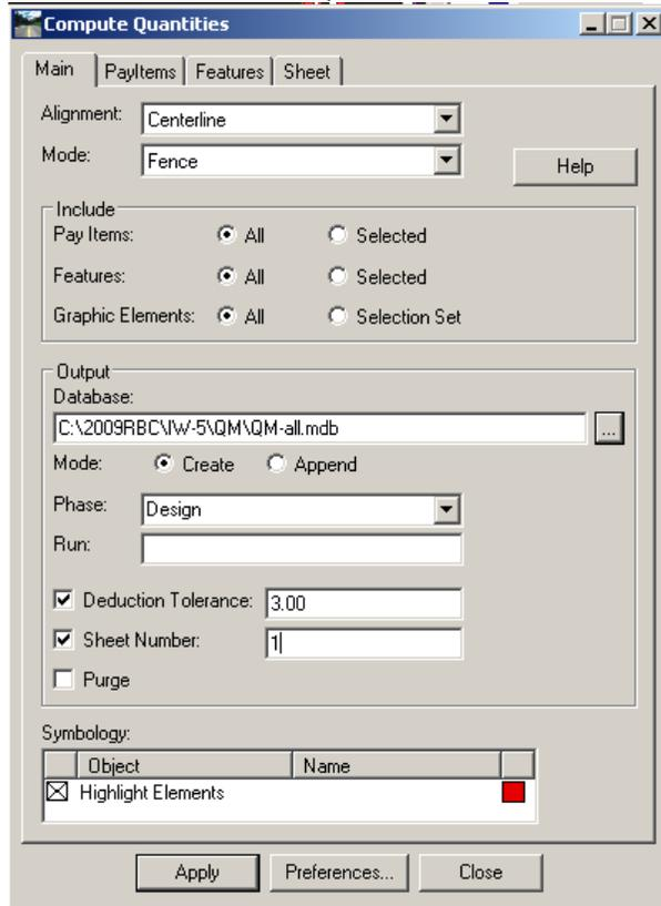
Set the output to the current working directory, make sure mode is set to Create, and toggle on the Sheet Number (1). For include, select All on each category.
