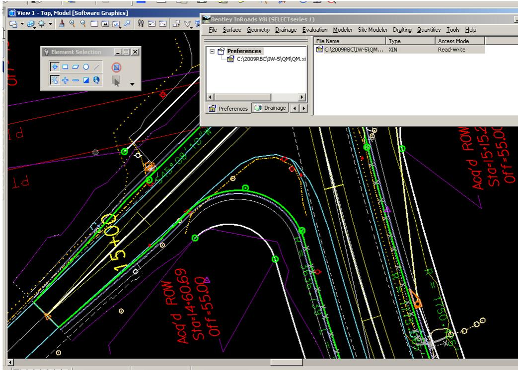
2. Place a Smartline as shown (any location will work). This is to represent a guardrail. Level/Symbology is not important.
