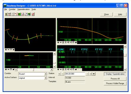
3. To set up super elevation we must first calculate the superelevation rates. **Right click** on the superelevation diagram pane and select **Create Superelevation Wizard>AASHTO**. This will bring up the **AASHTO Wizard**.
