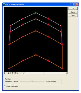
7. The reason nothing is happening is because of the constraints on the template points. To modify the constraints **right click** on the right lane line point and select **Edit point**.
