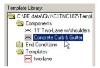
Holding the left mouse button down, drag the component onto the graph and rightclick (still holding down the left mouse button)
