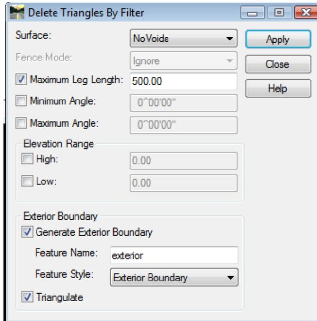
*Note:* This tool created an Exterior Boundary based on a Maximum triangle length of 500 feet in one step....any of the setting can be used in conjunction with each other to handle more complex analysis quickly.
