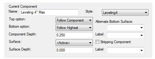
Note that you are setting the depth to 3" because 1" of leveling(the known minimum) is already part of the component. The template should look like this:
