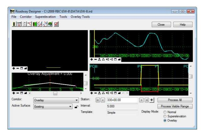
2. Switching to this mode activates the **Overlay Tools** commands. From the **Roadway Designer** menu, select **Overlay Tools** > **Cross Slope Optimization**.
