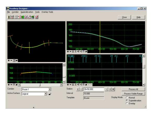
To set up super elevation we must first calculate the superelevation rates. Right click on the superelevation diagram pane and select Create Superelevation Wizard > AASHTO. This will bring up the AASHTO Wizard.
