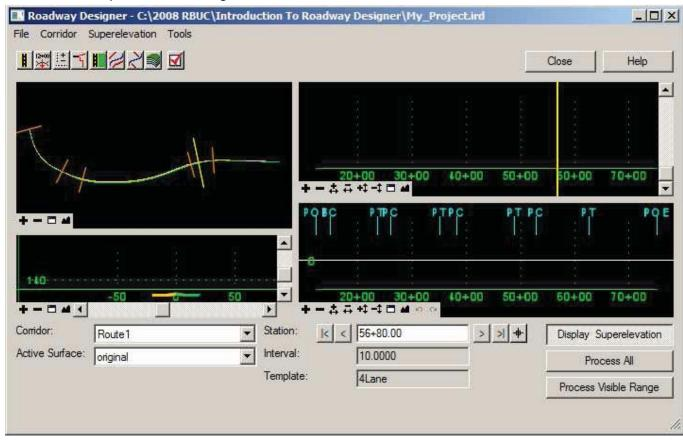
To set up superelevation we must first calculate the superelevation rates. Right click on the superelevation diagram pane and select Create Superelevation Wizard > AASHTO. This will bring up the AASHTO Wizard.
