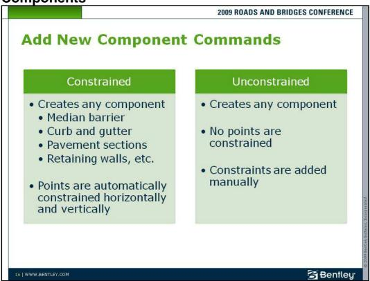
**Add New Component > Constrained** is used to create open and closed shaped template components using precision input. You can access this command by either right-clicking on the Current Template window or selecting it from the pull-down menu.
