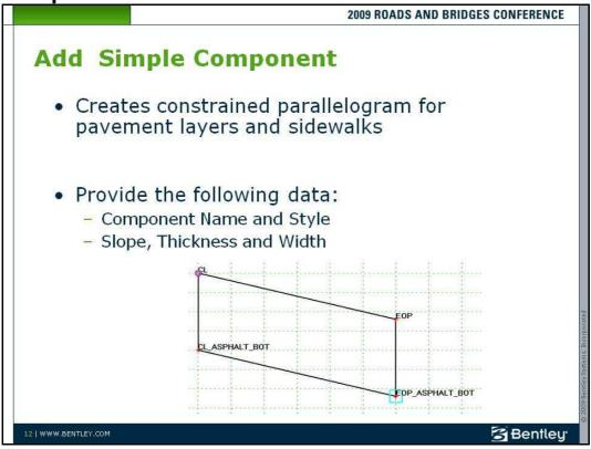
A component is a set of points that define an open or closed shape. Each component, whether open or closed, can represent a different material or area of interest.
