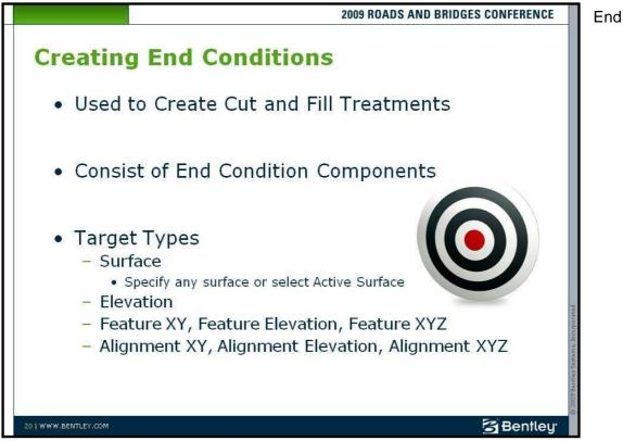
conditions are template components which are used to model cut and fill treatments. They are added to the end of simple, constrained, and unconstrained components.
