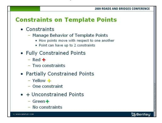
Point constraints are used to manage the behavior of template points. They are used so that if a point is moved in a template, either by you editing the template or by the application of point controls during design processing, all the points related to the point being moved will behave in a predictable manner.
