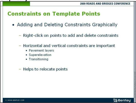
In addition to editing the template point constraints using the Point Properties dialog, you can right-click on any point to access **Add Constraint** or **Delete Constraints**. This is very handy for making quick adjustments to the template constraints.
