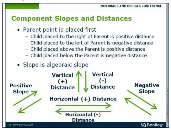
When defining components with precision input, the sign of the distance is dependent on the parent-child relationship. The parent is always the first point placed when creating template components. The distance is positive if the parent has a lower X or Y value than the child. The distance is negative if the parent has a higher X or Y value than the child. The sign of the component slope is based on the mathematical slope.
